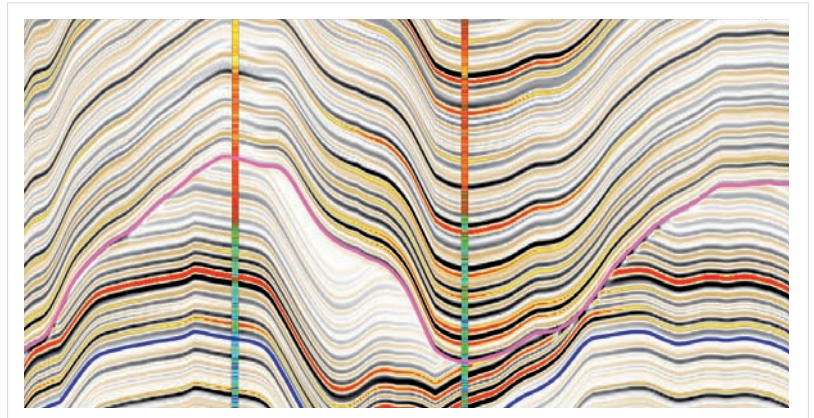
Synthetic model built using well logs, horizons and stratigraphic conformability constraints.
